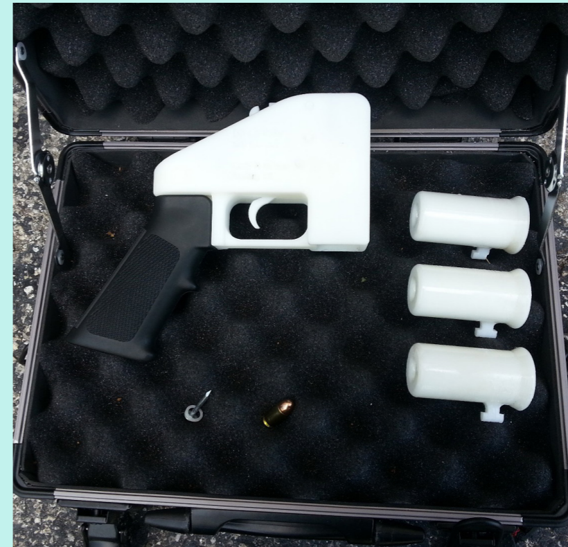
FIGURE 3.2. A WORKING GUN MADE FROM PLASTIC ON A 3D PRINTER 165
